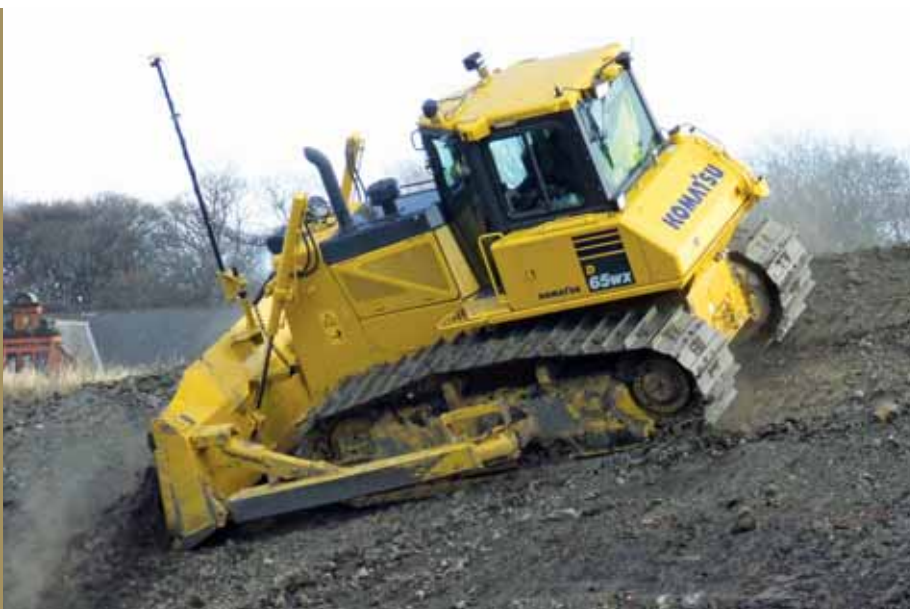
LEFT: Bulldozers were amongst the first machines to use GPS control technology
